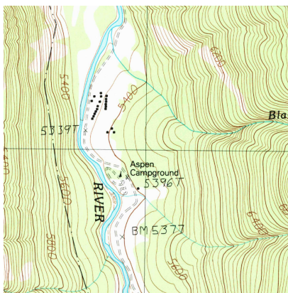
Figure 13.1.7 A topographical map displays elevation by drawing contour lines, along with the elevation is constant. USGS 1:24000-scale Quadrangle for Chrome Mountain, MT 1987.
