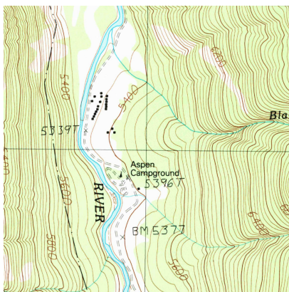
Figure 13.1.6 A topographical map displays elevation by drawing contour lines, along with the elevation is constant. USGS 1:24000-scale Quadrangle for Chrome Mountain, MT 1987.
