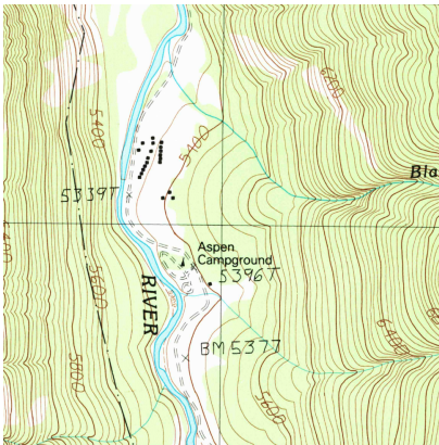
Figure 13.1.3: A topographical map displays elevation by drawing contour lines, along with the elevation is constant. Sample taken from the public domain USGS Digital Raster Graphics, http://topmaps.usgs.gov/drg/ .
